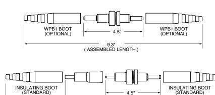
\_\_\_\_\_ 5.4" \_\_\_\_\_ ( ASSEMBLED LENGTH )
