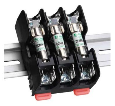
Littelfuse Class CC, G and Midget fuse blocks have integral DIN rail mounting capabilities that allow secure mounting to 35mm "hat" type DIN rails. This new releasable mechanism allows installation and removal of block without removing adjacent components on the DIN rail. Electrical panel builders and machine builders no longer need to use mounting adapters, saving assembly time and related costs.
