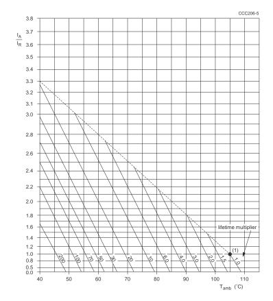
$I_A$  = actual ripple current at 100 Hz  $I_R$  = rated ripple current at 100 Hz and 105 °C
