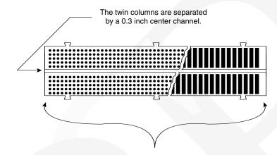
Each column has 64 groups of 5 connected terminals with 0.1 inch grid spacing.
