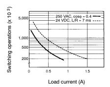
Reference: A maximum current of 0.5 A can be switched at 125 VDC (cosφ = 1).
