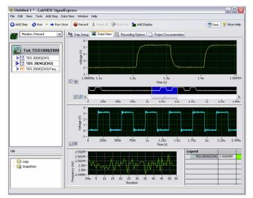
Easily capture, save, and analyze measurement results with included National Instrument's LabVIEW SignalExpress, Limited Tektronix Edition software.
