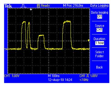
Data Logging enables automatic saving of triggered waveforms for up to 8 hours.
