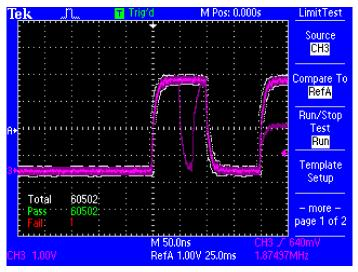
Limit Test provides a quick pass/fail comparison of any triggered input signal to a user-defined template.
