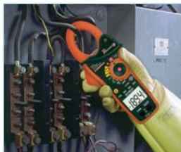
CAT IV -600V safety rating for added protection and True RMS feature gives you accurate readings of non-sinusoidal waveforms.
