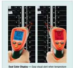
exceeds user programmed MAX and MIN setpoints, the display flashes from Blue to Red. Red backlit display will continue to flash until normal temperature is reached.
