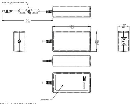
1.76" (H) x 3.13" (W) x 5.87" (L) 44.0 mm (H) x 79.6 mm (W) x 149.0 mm (L) AC Input Connector: IEC320, C14 AC Input power cord sold separately
