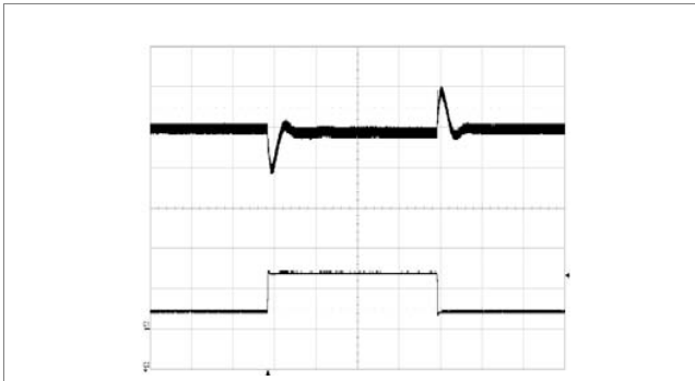
Output voltage response to load current step-change (5-15-5 A) at: T_{P1} = +25^\circ\text{C} , V_i = 12\text{ V} , C_o = 1.8\text{ mF} . Top trace: output voltage (200 mV/div.). Bottom trace: load current (10 A/div.). Time scale: (0.5 ms/div.).
