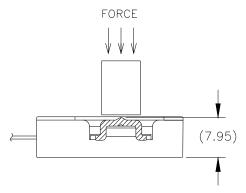
LOAD MUST ONLY BE APPLIED TO THE CONCENTRATOR TIP IN THE CENTER OF THE SENSOR TO MAINTAIN ACCURACY
