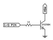
Switching circuit for the Propeller chip. Note: HIGH signal is required to turn on heater due to inversion of signal by the transistor.
