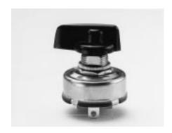
The 700-Series rotary switches are AC/ DC rated, multi-position, single pole switches. These switches feature a nylon actuator and shaft in a metal clad construction. The 700-Series also feature a self-cleaning wiping action and a silverplated contact system.
