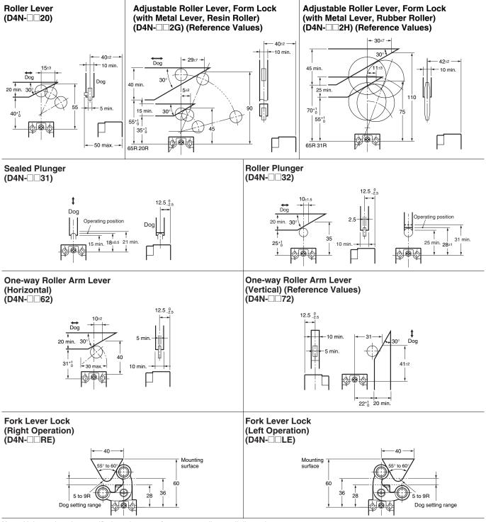
Note: Unless otherwise specified, a tolerance of  $\pm 0.4$  mm applies to all dimensions.
