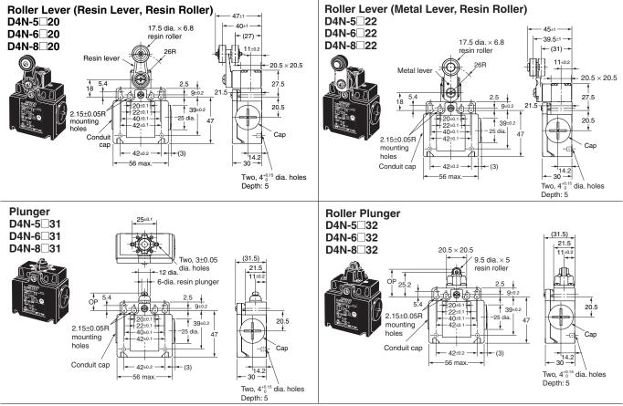
**Note:** Unless otherwise specified, a tolerance of  $\pm 0.4$  mm applies to all dimensions.
