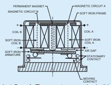
snap it into a closed position against Core A. The armature remains in this position upon removal of power from Coil B, but will snap back into position B upon energizing Coil A. Since operation depends upon cancellation of a magnetic field, it is necessary to apply the correct polarity to the relay coils as indicated on the relay schematic.
