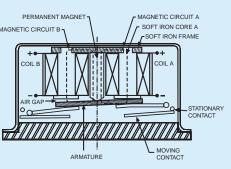
snap it into a closed position against Core B. The armature remains in this position upon removal of power from Coil A, but will snap back into position A upon energizing Coil B. Since operation depends upon cancellation of a magnetic field, it is necessary to apply the correct polarity to the relay coils as indicated on the relay schematic.
