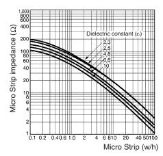
• For example, when creating  $50-\Omega$  lines using a glass epoxy base with a thickness of 1.6 mm, the above graph will yield a w/h ratio of 1.7 for a dielectric constant of 4.8. Since the base thickness is 1.6 mm, the width will be h × 1.7  $\approx$  2.7 mm.
