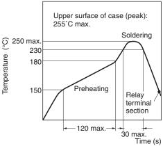
**Note:** The temperature profile indicates the temperature of the relay terminal section.
