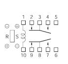
Single coil latch type (reset position)
