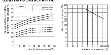
Note: The maximum coil voltage refers to the maximum value in a varying range of operating power voltage, not a continuous voltage.
