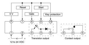
Note: 1 and 6 are connected to each other internally.
