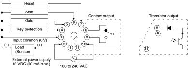
Note: Power supply circuit is insulated from the internal circuit (or I/C
