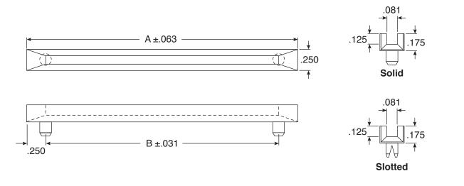
Printed circuit board support guides are an economical and fast solution to mount P.C. Boards. Card insertion is simple and fast. The smooth positive channel guides the P.C. Board and firmly supports and protects the board. Guides are molded of tough, electrically insulating nylon 6/6 and are designed to snap into pre-punched holes in the chassis.
