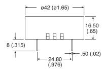
Piezoelectric Buzzer (Built-In Drive)
