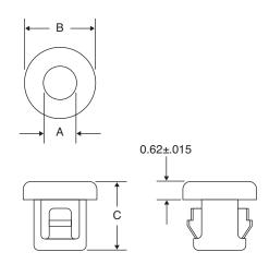
EPD bushings provide economical protection for wire, cable, tubing, and hose from sharp, uneven drilled or punched holes in sheet metal.
