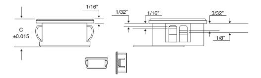
These bushings are available in a large selection of sizes from 1/4" to 2" in various inside diameter openings. Standard bushing are designed with multiple locks to positively snap in panels ranging from 1/32" to 1/8" thickness.
