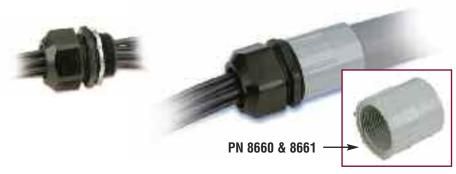
Use of the Heyco Solar Masthead, Heyco-Flex I (page 2-1) or rigid PVC conduit, and the Heyco Coupling allows the installer to run PV wire output hookup off the rooftop and connect to field level inverter.
