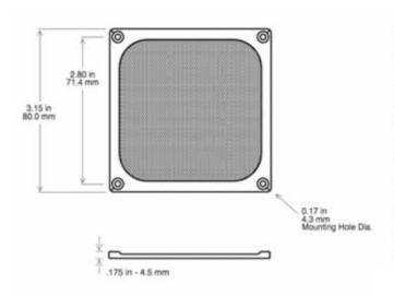
Aluminum/Stainless filters offer high levels of air passage while efficiently filtering contaminants and shielding EMI/RFI.
