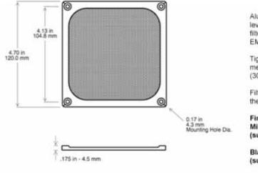
Aluminum/Stainless filters offer high levels of air passage while efficiently filtering contaminants and shielding EMI/RFI.
