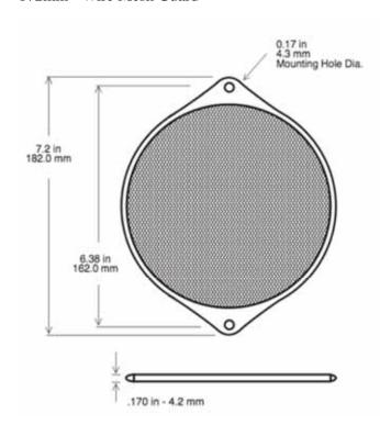
Aluminum/Stainless filters offer high levels of air passage while efficiently filtering contaminants and shielding EMI/RFI.
