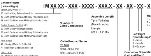
B0= Matte Sn Plating, Straight Solder Tail B1= Matte Sn Plating, Retention Solder Tail
