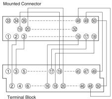
Terminal Block Note: Connector pin numbers correspond 1-to-1 to terminal block numbers on all models.
