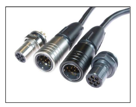
The PPS is a miniature connector with push pull technology and RoHS compliant. It is designed for use on equipment that is not submersed or left exposed to the elements for prolonged periods, within Industrial and Ground Harsh Environment applications. To mate, the plug is pushed onto the receptacle. The connector is locked in its rest position and is released by pulling back the coupling nut.
