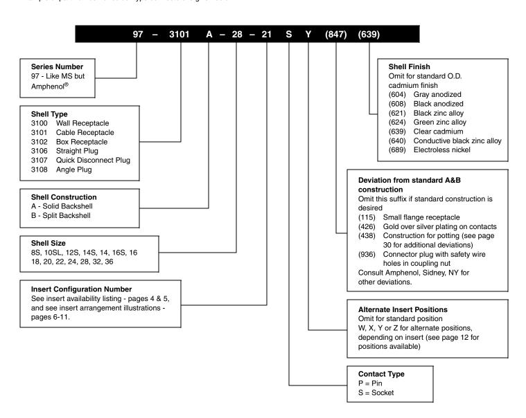
Note: Accessories for 97 Series Connectors should be ordered with matching connector plating. See accessory pages 33-39.
