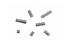
PRA arrays can be used in most applications requiring a matched pair (or set) of resistor elements. The networks provide 1 ppm/°C TCR tracking, a ratio tolerance as tight as 0.01 % and outstanding stability. They are available in 1 mm, 1.35 mm and 1.82 mm pitch.
