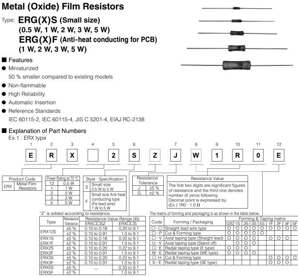
The above example 1 shows a small metal film resistor, 2 W power rating, resistance value of 1.0  $\Omega$ , tolerance ±5 %, and package of radial taping.
