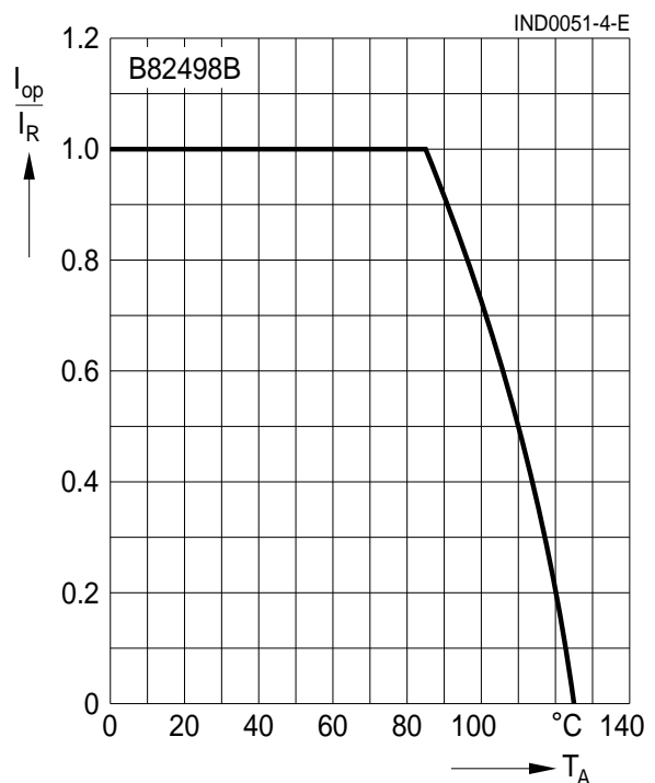
Current derating I op /I R versus ambient temperature T A (rated temperature T R = 85 °C)
