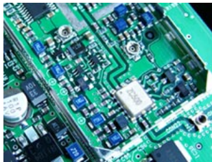
Applicational example of NL series: ETC on-board unit (Signal lines of receiving circuit)
