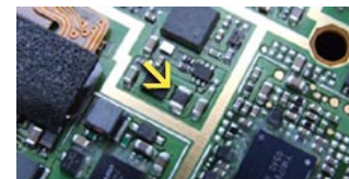
Applicational example of GLF series: Vcc lines of cellular phone
