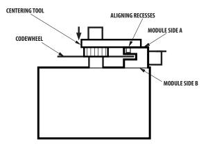
Figure 3. Alignment Tool is Placed over Shaft and onto Codewheel Hub. Alignment Tool Pins Mate with Aligning Recesses on Module.
