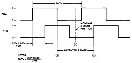
CHANNEL A LEADS CHANNEL B FOR CLOCKWISE ROTATION
