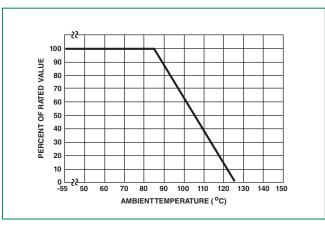
For applications exceeding  $85^{\circ}$  C, ambient temperatures, the peak surge current and energy rating must be reduces as shown in Figure 1.
