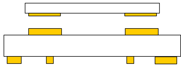
Figure 20. Correct PCB Top Metal Pattern Under Package
