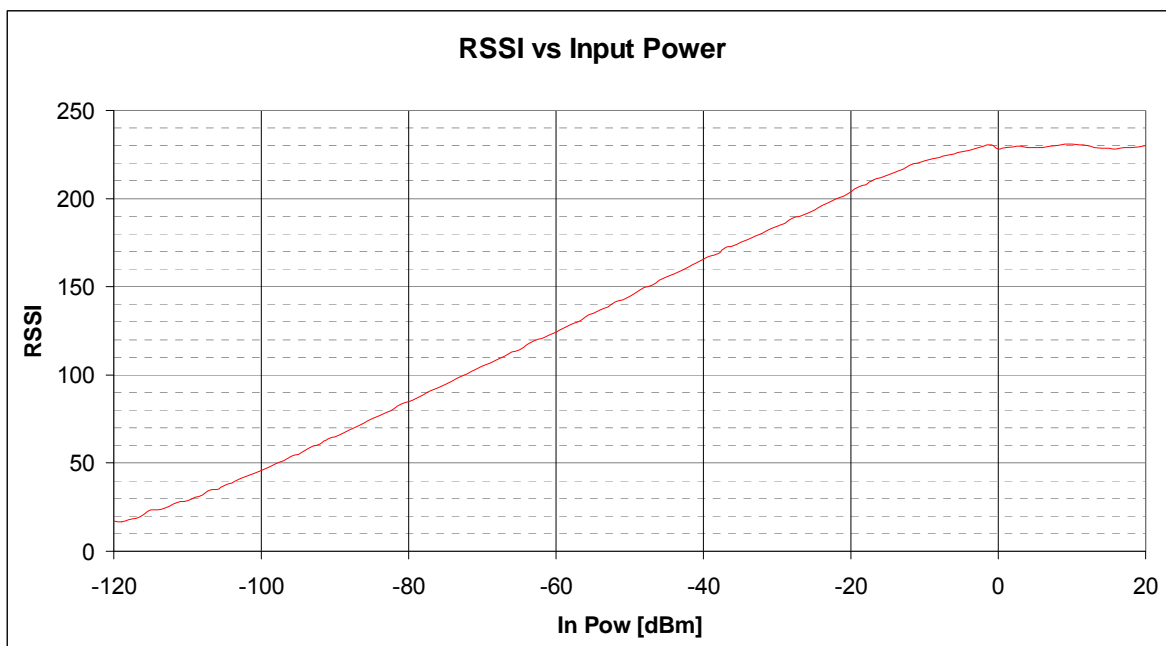
Figure 23.25. RSSI Value vs. Input Power
