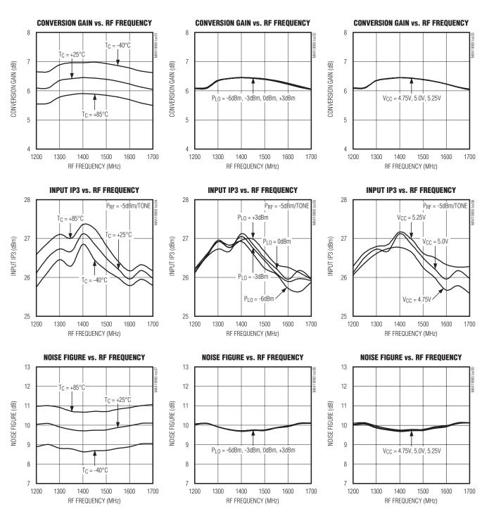
(*Typical Operating Characteristics (continued*) (*Typical Application Circuit* (see Table 1). Vcc = 5.0V, f<sub>RF</sub> > f<sub>LO</sub> for a 140MHz IF, P<sub>RF</sub> = -5dBm, P<sub>LO</sub> = 0dBm, T<sub>C</sub> = +25°C, unless otherwise noted.)
