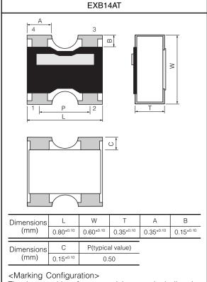
The bar marking for recognizing terminal direction is located on the side of terminal 3, 4. Mass (Weight) [1000 pcs.] : 0.7 g
