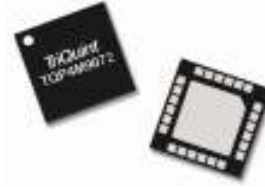
24-pin 4x4mm leadless QFN package
