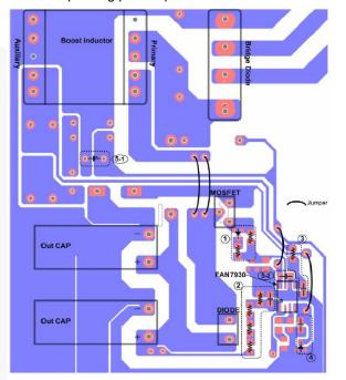
Figure 43. Recommended PCB Layout
