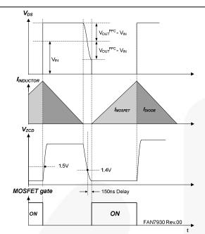
Figure 28. Auxiliary Voltage Threshold
