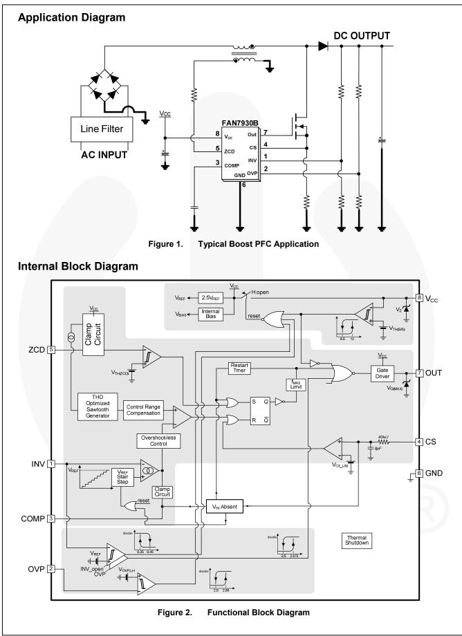
FAN7930B — Critical Conduction Mode PFC Controller
