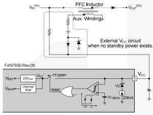
Figure 22. Startup Circuit
