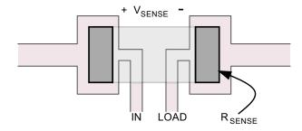
Choose a low inductance type sense resistor if preservation of bandwidth is important. The use of Kelvin connections helps by excluding the inductive voltage drop across the traces leading to the sense resistor. The inductive voltage drop may be substantial when operating at high frequencies. A trace or component inductance of just 10nH contributes an impedance of  $6.2 m\Omega$  at 100 kHz, which constitutes a 6% error when using a  $100 m\Omega$  sense resistor.
