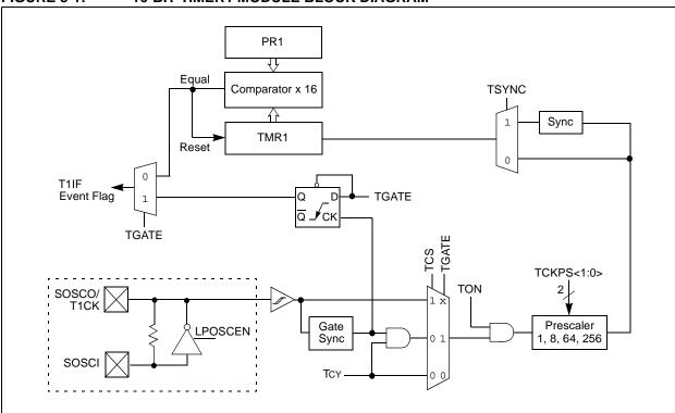
FIGURE 8-1: 16-BIT TIMER1 MODULE BLOCK DIAGRAM
