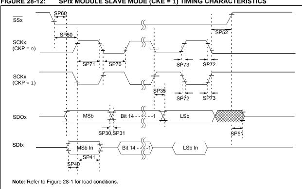
SPIX MODULE SLAVE MODE (CKE = 1) TIMING CHARACTERISTICS FIGURE 28-12:
