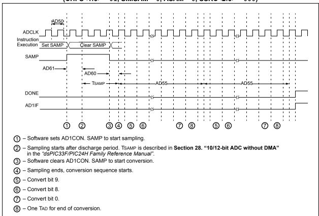
**FIGURE 28-20:** ADC CONVERSION (10-BIT MODE) TIMING CHARACTERISTICS (CHPS<1:0> = 01, SIMSAM = 0, ASAM = 1, SSRC<2:0> = 111, SAMC<4:0> = 00001)
