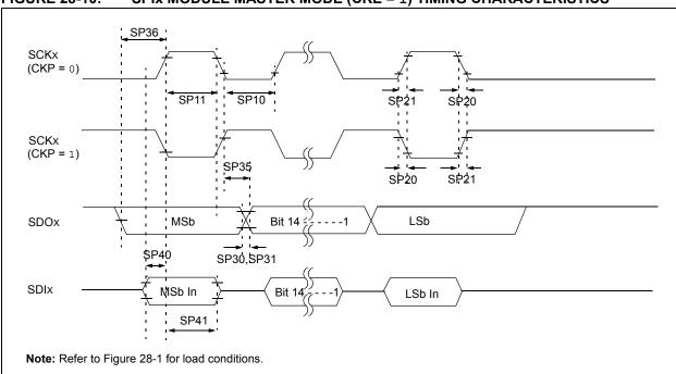
FIGURE 28-10: SPIX MODULE MASTER MODE (CKE = 1) TIMING CHARACTERISTICS
