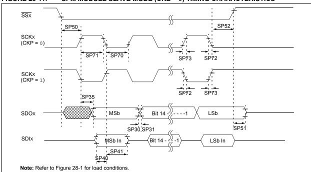
FIGURE 28-11: SPIX MODULE SLAVE MODE (CKE = 0) TIMING CHARACTERISTICS
