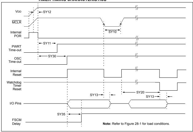
TABLE 28-21: RESET, WATCHDOG TIMER, OSCILLATOR START-UP TIMER, POWER-UP TIMER TIMING REQUIREMENTS
