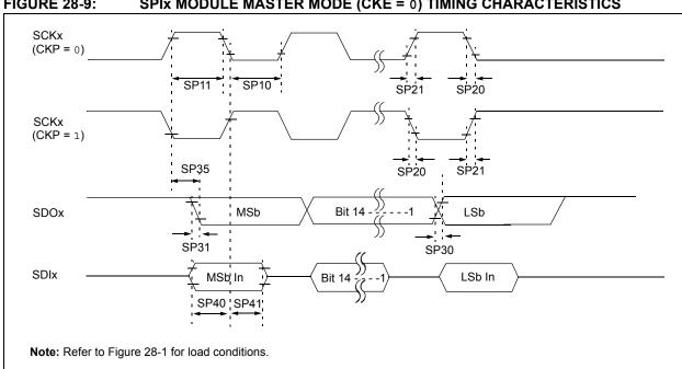
**FIGURE 28-9:** SPIX MODULE MASTER MODE (CKE = 0) TIMING CHARACTERISTICS
