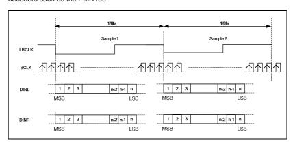
Figure 19 8FS Mode Left Justified Timing Requirements
