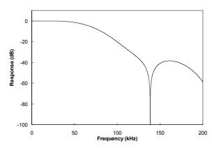
Figure 60 DSD Plus Mode Filter 1 Frequency Response
