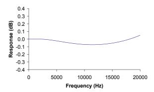
Figure 80 De-emphasis Frequency Response (48kHz)
