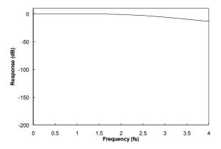
Figure 58 8FS Mode Filter Frequency Response
