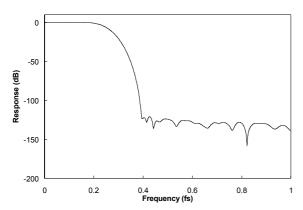
Figure 54 High Rate PCM Filter 4 Frequency Response
