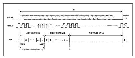
Figure 18 DSP Mode B Timing Diagram
