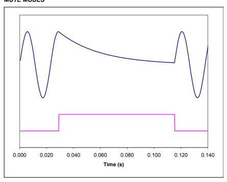
Figure 24 Application and Release of Soft Mute
