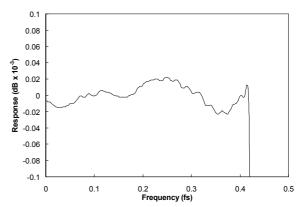
Figure 31 Low Rate PCM Filter 2 Ripple
