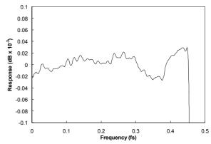
Figure 33 Low Rate PCM Filter 3 Ripple
