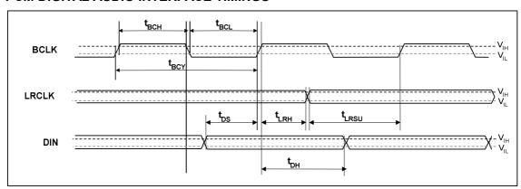
Figure 2 Digital Audio Data Timing
