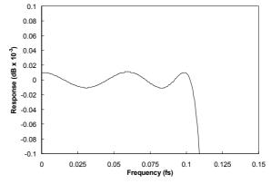
Figure 48 High Rate PCM Filter 1 Frequency Response
