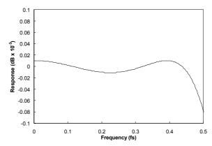
Figure 59 8FS Mode Filter Ripple
