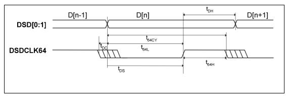
Figure 3 DSD Audio Timing - Normal Mode
