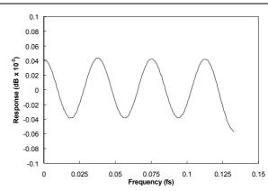
Figure 53 High Rate PCM Filter 3 Ripple
