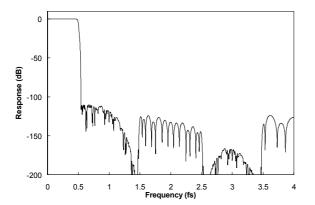
Figure 32 Low Rate PCM Filter 3 Frequency Response
