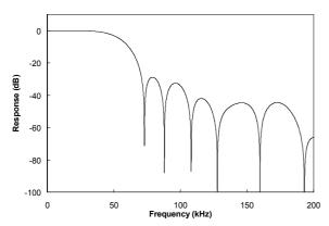
Figure 62 DSD Plus Mode Filter 2 Frequency Response
