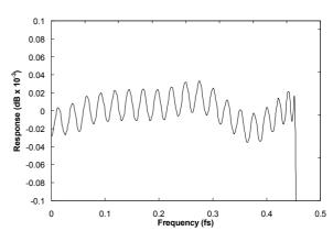
Figure 29 Low Rate PCM Filter 1 Ripple
