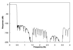
Figure 36 Low Rate PCM Filter 5 Frequency Response
