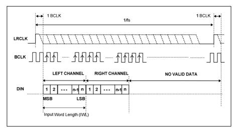
Figure 17 DSP Mode A Timing Diagram
