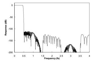
Figure 34 Low Rate PCM Filter 4 Frequency Response
