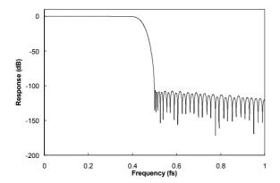
Figure 52 High Rate PCM Filter 3 Frequency Response
