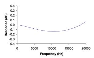
Figure 78 De-emphasis Frequency Response (44.1kHz)
