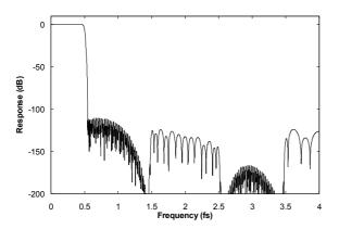
Figure 28 Low Rate PCM Filter 1 Frequency Response
