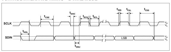
Figure 6 Control Interface Timing - 2-Wire Serial Control Mode
