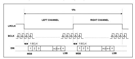
Figure 16 I<sup>2</sup>S Mode Timing Diagram
