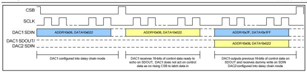
Figure 11 Initial Setup of Two WM8741 Devices into Control Interface Daisy Chain Mode
