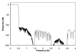
Figure 30 Low Rate PCM Filter 2 Frequency Response
