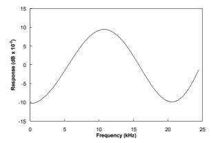
Figure 64 DSD Plus Mode Filter 3 Frequency Response
