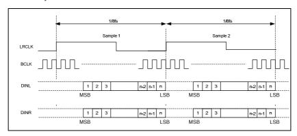
Figure 20 8FS Mode Right Justified Timing Requirements
