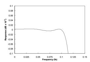
Figure 50 High Rate PCM Filter 2 Frequency Response
