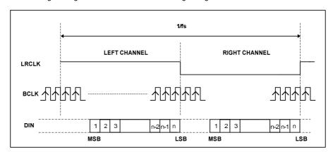
Figure 15 Right Justified Mode Timing Diagram
