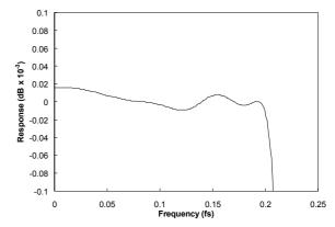
Figure 40 Medium Rate PCM Filter 2 Frequency Response
