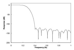
Figure 56 High Rate PCM Filter 5 Frequency Response
