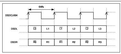
Figure 23 Bi-phase DSD Mode Timing Diagram
