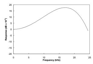
Figure 74 DSD Direct Mode 8fs Notch High Gain Filter Frequency Response
