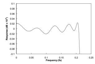
Figure 46 Medium Rate PCM Filter 5 Frequency Response
