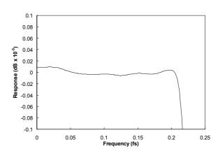
Figure 44 Medium Rate PCM Filter 4 Frequency Response
