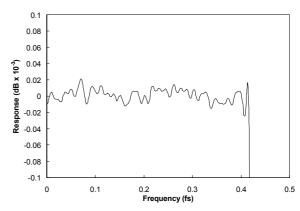
Figure 37 Low Rate PCM Filter 5 Ripple
