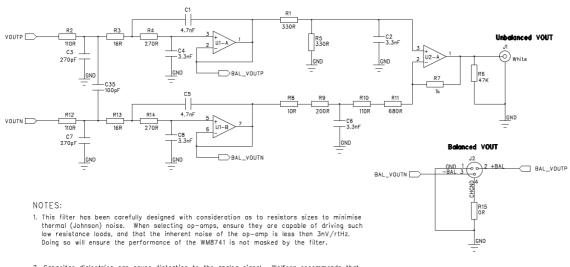
Capacitor dielectrics can cause distortion to the analog signal. Wolfson recommends that multilayer ceramic capacitors be used, with dielectric material COG or NPO for optimum performance.
