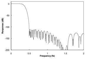
Figure 38 Medium Rate PCM Filter 1 Frequency Response
