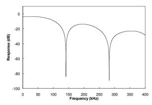
Figure 68 DSD Direct Mode Standard Low Gain Filter Frequency Response
