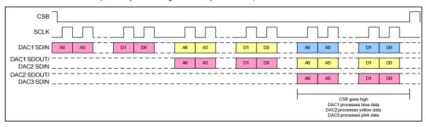
Figure 12 Daisy Chain Control Interface Example for Three WM8741 Devices
