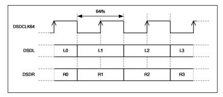
Figure 22 Uni-phase DSD Mode Timing Diagram
