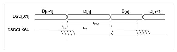
Figure 4 DSD Audio Timing - Phase Modulated Mode
