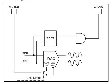
Figure 27 Hardware Control Mode MUTEB and ZFLAG Configuration
