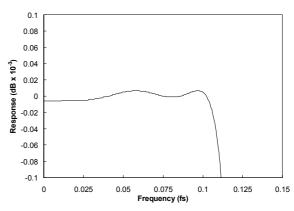
Figure 55 High Rate PCM Filter 4 Ripple
