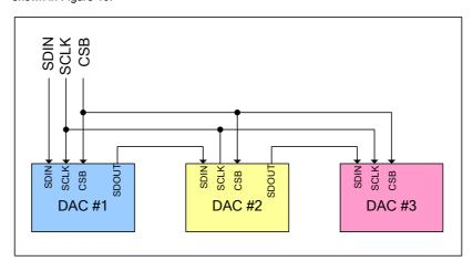
Figure 10 Control Interface Daisy Chaining Setup
