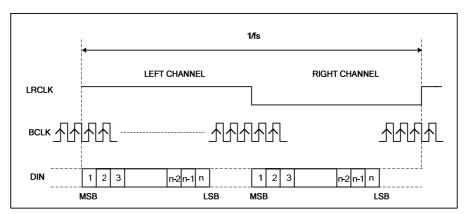
Figure 14 Left Justified Mode Timing Diagram
