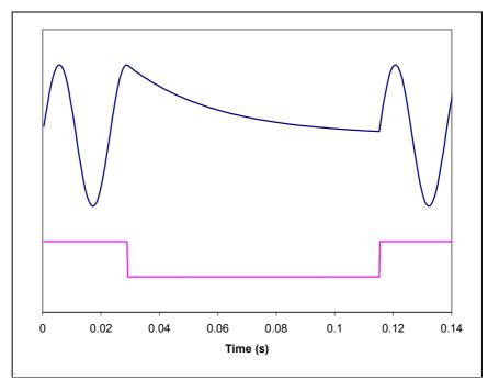
Figure 26 Hardware Control Mode Soft Mute Characteristic
