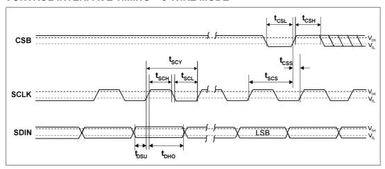
Figure 5 Control Interface Timing - 3-Wire Serial Control Mode
